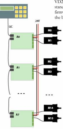
VD203 is used in two basic configurations : master/slave and standalone. Off the shelf, the board is shipped with slave firmware. When assembling master/slave systems, grounding the boards is a critical issue. The problem arises from the
