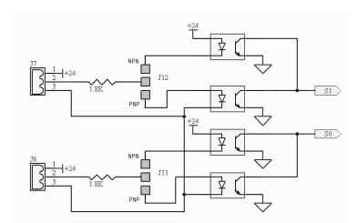
The inputs accept optical or magnetic sensors with either PNP or NPN outputs. The sensor type is configured by J11 and J12.
