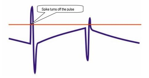
These spikes fool the current limit circuitry into thinking that the limit has been reached and turn off the PWM pulse prematurely. The result is that the PWM stays at minimum duty cycle and the motor barely moves or doesn't move at all.
