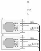
There are two RJ-45 I2C connectors wired in parallel. Having two connectors allows to daisy-chain multiple boards.
